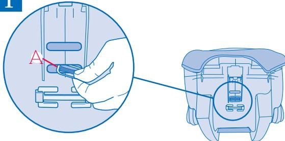
To reposition the crotch strap, turn the harness anchor **A** on the end of the crotch strap sideways and push it through the slot in the restraint seat.
