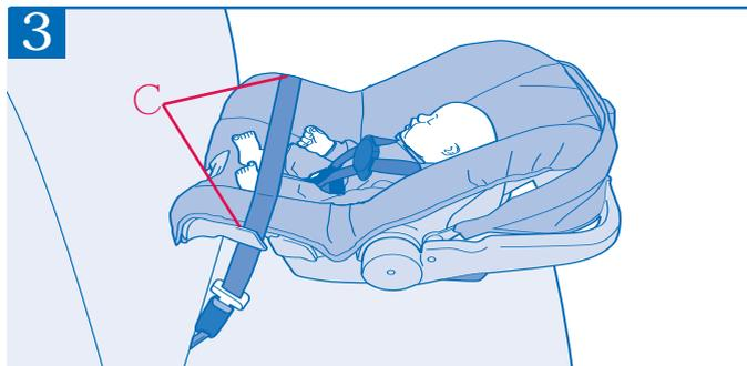
Secure the restraint to your vehicle by routing the vehicle seat belt through the belt slots **C** on the sides of the restraint.
