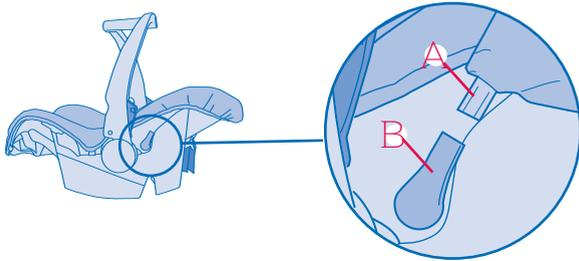
Guide each end of the canopy strip **A** into the canopy holders **B** located on each side of the child restraint.
