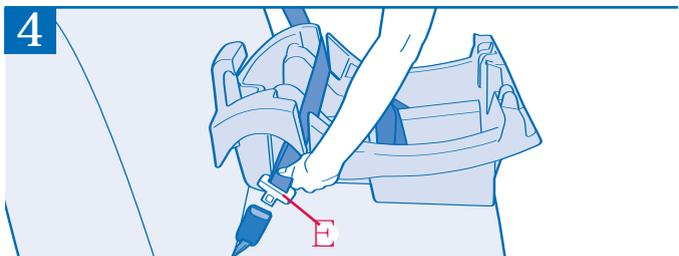
Hold the lap and shoulder belts together just behind the free sliding buckle tongue **E** and unbuckle the seat belt.
