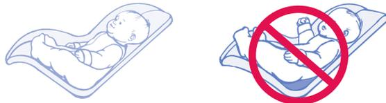
Dress your infant in clothing with legs. The harness must pass between the baby's legs, clothing with legs allows a better fit. Do not use a sack sleeper or a bulky blanket. Place your infant 5 to 22 lbs (2.3 to 10 kg), 19 to 29 inches (48 to 74 cm) in the restraint. Baby's back and bottom should be flat against the seat. If you leave a gap, baby will not be comfortable.
