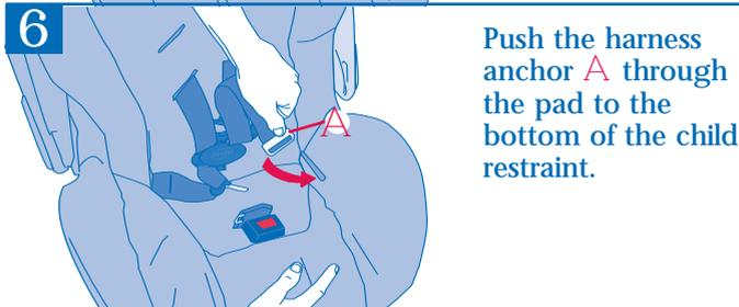
Push the harness anchor **A** through the pad to the bottom of the child restraint.
