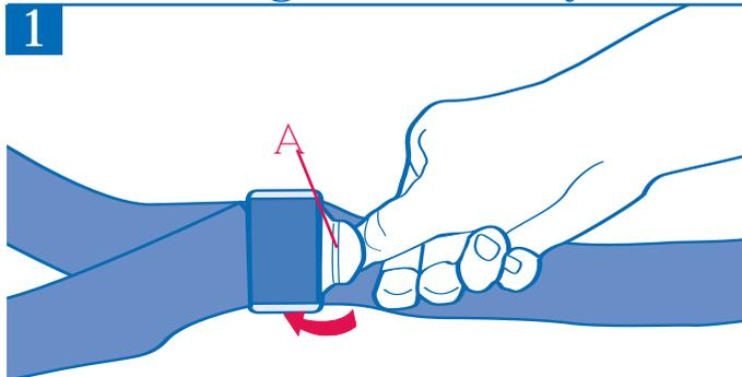
Tilt and slide the adjuster **A** to loosen.
