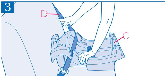
Push down on the base **C** while pulling the shoulder belt **D** tightly to remove all slack from the lap portion of the belt.
