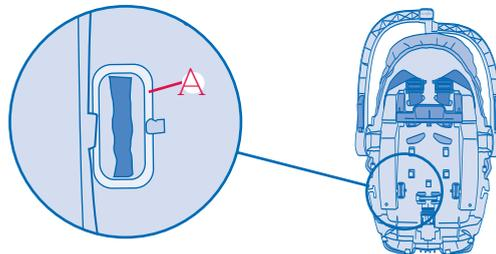
Pull the harness anchor **A** through the bottom of the child restraint, and clip into place. Repeat on the opposite side.
