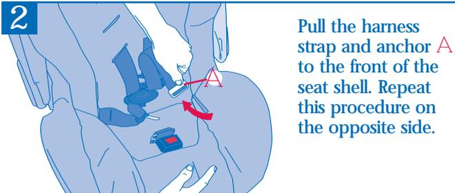
Pull the harness strap and anchor **A** to the front of the seat shell. Repeat this procedure on the opposite side.
