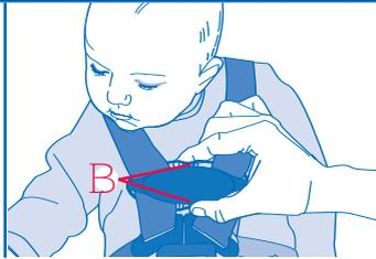
To unfasten the chest clip, squeeze the tabs **B** together and pull the clip apart.
