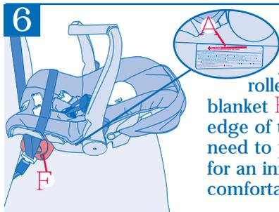
If the level line **A** is not level to the ground, use a tightly rolled towel or small blanket **F** beneath the front edge of the child restraint. You need to provide enough recline for an infant's head to lie back comfortably.
