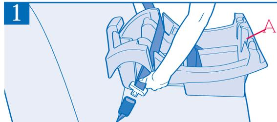
Secure the base **A** to your vehicle seat by routing the vehicle seat belt through the openings on the sides of the base. You may also let the vehicle shoulder belt fall against the vehicle seat back. Be sure that the vehicle shoulder belt does not lie inside any portion of the convenience base.
