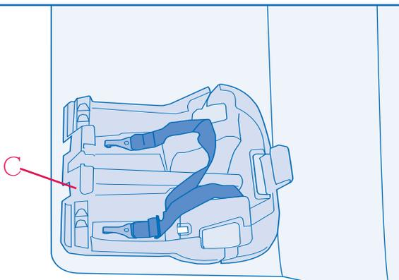
When the LATCH system is not in use, you **MUST** securely store it in the area provided in the base **C**. Fold the harness strap, place it in the middle, and put the hooks in the slots located on each side of the storage area. A loose LATCH harness and hook may injure your child.
