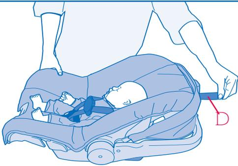
Tighten the harnesses by pulling on the harness straps **D** from the back of the harness adjusters.
