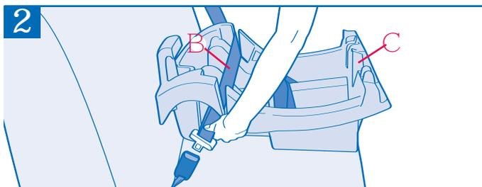
Thread the seat belt **B** through the base **C** (or child restraint) and buckle the seat belt.
