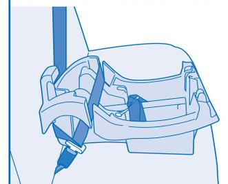
NOTE: In vehicles with a lap and shoulder belt **and** a **free-sliding buckle tongue**, you **MUST** install with the locking clip. See “Using the Locking Clip” on page 23.
