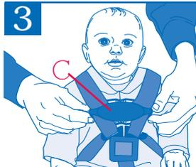
Align the two sides of the chest clip **C** and snap them together. The chest clip must be positioned at armpit level.
