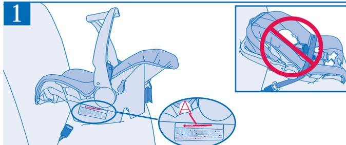
After securing the infant, place the restraint into your vehicle. Adjust the restraint so that the level line **A** is parallel with the vehicle floor.
