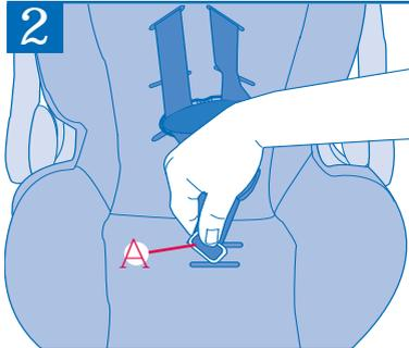
Insert the crotch strap anchor **A** into the slot that is closest to the child **AND** the most comfortable for the child.
