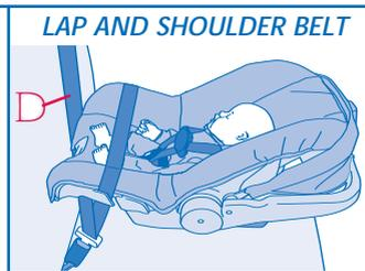
**NOTE:** In vehicles with a lap and shoulder belt **D** and a free sliding buckle tongue, and emergency locking retractors (ELR) you must install with the locking clip. Unless your vehicle owner's manual provides otherwise. See "Using the Locking Clip" on page 23.
