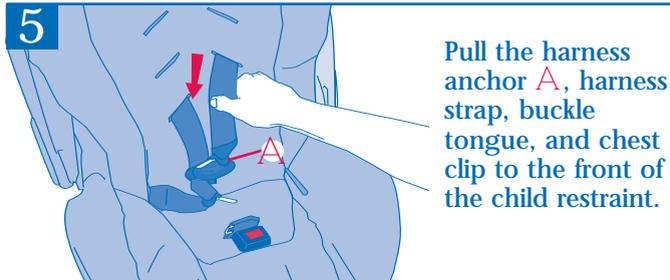
Pull the harness anchor **A**, harness strap, buckle tongue, and chest clip to the front of the child restraint.
