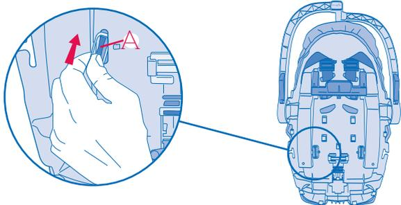
Push the harness anchor **A** located on the back of the child restraint through the slot to the front of the seat shell. Repeat this procedure on both sides.
