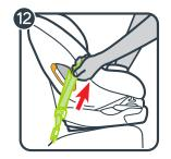
12. Remove lower anchor strap slack. Press down firmly in the center of the car seat while tightening the lower anchor strap. You may need to tighten through the slit in the pad at the belt path as shown.
