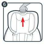
6. Squeeze the headrest adjustment handle and raise the headrest to the highest position.
