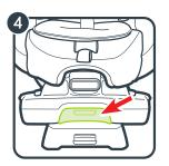
4. From the front of the car seat, open the lower anchor storage door. Remove the lower anchor strap and connectors from the storage compartment. Close the lower anchor storage door
