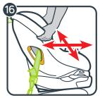
16. Test for tightness. Grab the sides of the seat where the lower anchor strap is and slide the car seat side to side and front to back. If the seat moves less than 1" (2.5 cm), it is tight enough.
