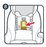
8. Open the RAPIDLOCK lock-off by pushing the gray button and lifting the lock-off arm.
