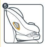
4. Unhook the tether from the storage location on the back on the seat, and lay it over the front of the seat.
