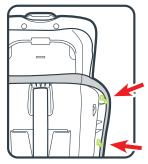
Remove the edges of the pad fabric from the 4 clips found inside the car seat shell lip
