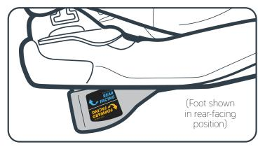
Unsnap the foot from base by pulling on the foot. Swing the foot forward or back to change positions. The recline foot is secure when it "clicks" into place.
