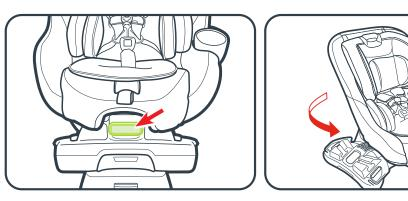
For rear-facing installation the car seat MUST be rotated to access rear facing belt path marked with a blue stripe.
