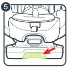
5. From the front of the car seat, open the lower anchor storage door. Remove the lower anchor strap and connectors out of the storage compartment. Close the lower anchor storage door
