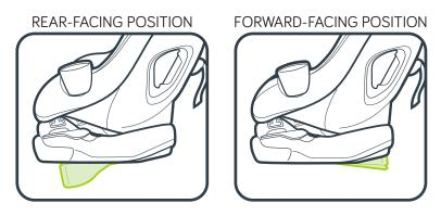
The correct position is marked with a label on the side of the foot. The foot is correctly in the rear-facing position with the blue text is facing up. The foot is correctly in the forward-facing position with the orange text is facing up.
