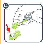
13. When the slack is removed, close the RAPIDLOCK Lock-Off until you hear a "Click". Make sure the lower anchor strap is under the RAPIDLOCK Lock-Off.
