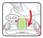
When the slack is removed, close the RAPIDLOCK Lock-Off until you hear a "Click". Make sure the vehicle seat belt or lower anchor strap is under the RAPIDLOCK Lock-Off.
