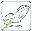
LOWER ANCHOR ATTACHMENT Do not install by this method for a child weighing more than 35 lb (16 kg)
