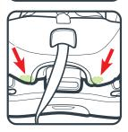
5. Check the buckle position. The correct slot is the one that is closest to your child without being underneath them.
