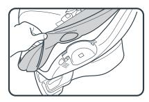
2. Align the tabs on the cup holder with the slots in the shell and insert the cup holder until you hear a "Click!"
