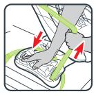
Remove vehicle seat belt or lower anchor strap slack. Press down firmly near the front of the base. (rear-facing installation with vehicle lap and shoulder belt shown).
