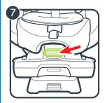
7. Squeeze the rotation lever at the front of the car seat and rotate the seat. The seat may be rotated towards or away from you.
