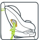
LOWER ANCHOR ATTACHMENT WITH TETHER STRAP Do not install by this method for a child weighing more than 40 lb (18kg)
