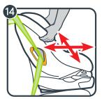
14. Test for tightness. Grab the sides of the seat where the vehicle seat belt is and slide the car seat side to side and front to back. If the seat moves less than 1" (2.5 cm), it is tight enough.
