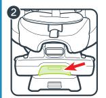
2. Store the lower anchor connectors inside the lower anchor storage compartment.
