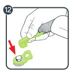
11. When the slack is removed, close the RAPIDLOCK lock-off until you hear a "Click". Make sure the vehicle seat belt is under the RAPIDLOCK Lock-Off.
