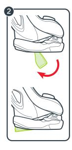
2. Rotate the recline foot on the bottom of the car seat into the forward-facing position marked with a orange label. The recline foot is secure when it "clicks" into place.
