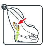
10 Thread the lower anchor strap through the orange forwardfacing belt path, through the RAPIDLOCK lock-off, and out the other side. The lower anchor strap should lie as flat as possible and not be twisted.
