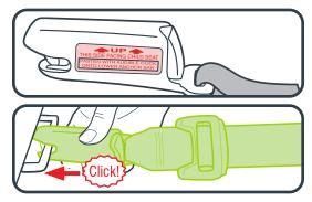
12. Remove lower anchor strap slack. Press down firmly near the front of the base while tightening the lower anchor strap.
