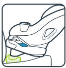
15. Check the level indicator. Vehicle MUST be on level ground. Bubble must be completely under the blue lines. Adjust the recline until the bubble is completely under the blue lines. For infants 3 months and under, the bubble must be entirely under the light blue line.
