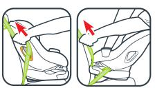
may start to tilt your car seat sideways. If this happens, use a locking clip instead of switching the retractor. See Sliding Latch Plate and ELR Retractor.
