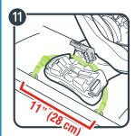
11. Attach the lower anchor connectors to the vehicle's lower anchors. Make sure the arrows are pointing up.
