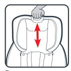
To raise or lower headrest/harness height, squeeze the adjustment handle and move headrest for the proper harness
