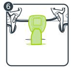
6. Replace seat pad, making sure the buckle goes through the same slot in the seat pad as in the plastic shell
