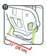
11. Attach lower anchor connectors to vehicle's lower anchors. Make sure the arrows are pointing up.
