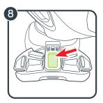
8. Open the RAPIDLOCK lock-off by pushing the gray button and lifting the lock-off arm.
