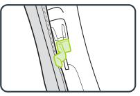
Remove the edges of the pad fabric from the ribs on lower sides of the seat.
