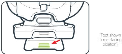
The foot has 3 recline positions. Always make sure to recheck the level indicator after adjusting the recline when using the seat in rear-facing mode.
