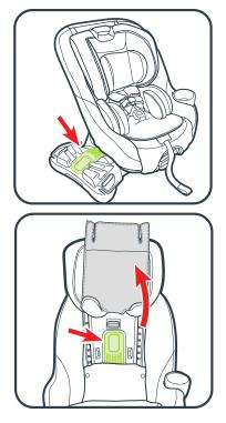
The rear-facing RAPIDLOCK is located on the base and can only be found by rotating the seat.
