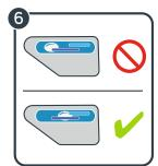
6. Check the level indicator. Vehicle **MUST** be on level ground. **Bubble must be completely under the blue lines.** Adjust the recline until the bubble is completely under the blue lines. For infants 3 months and under, **the bubble must be entirely under the light blue line.**
