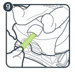
9. Tighten the harness by pulling the harness adjustment strap. A snug harness should not allow any slack. It lies in a relatively straight line without sagging. It does not press on the child's flesh or push the child's body into an unnatural position.
