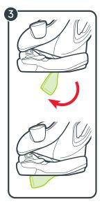
3. Rotate the recline foot on the bottom of the car seat into the rear-facing position marked with a blue label. The recline foot is secure when it "clicks" into place.
