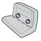
The child restraint's lower anchors are designed to be used at the standard lower anchor spacing of 11" (28 cm) from the center of one anchor point to the center of another anchor point. Please refer to your vehicle owner's manual for information about using lower anchors in certain seating positions.
