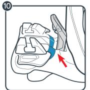
10. Route the lower anchor strap along the blue stripe across the base and under the RAPIDLOCK lock-off arm.
