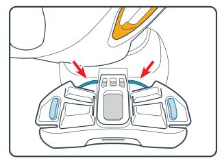
With your child secured, rotate the seat to the rear-facing position. The seat is secure when you hear a "CLICK!" Pull on the sides of the seat to make sure it is locked.
