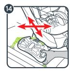
14. Test for tightness. Grab the sides of the base where the lower anchor strap is and slide the base side to side and front to back.
